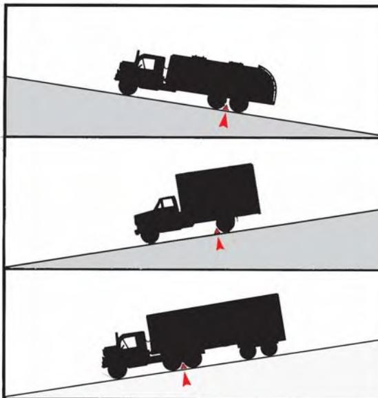
When parking on a hill, use chock blocks to reduce the chances of a runaway vehicle. Recommended placement of blocks indicated in red.
