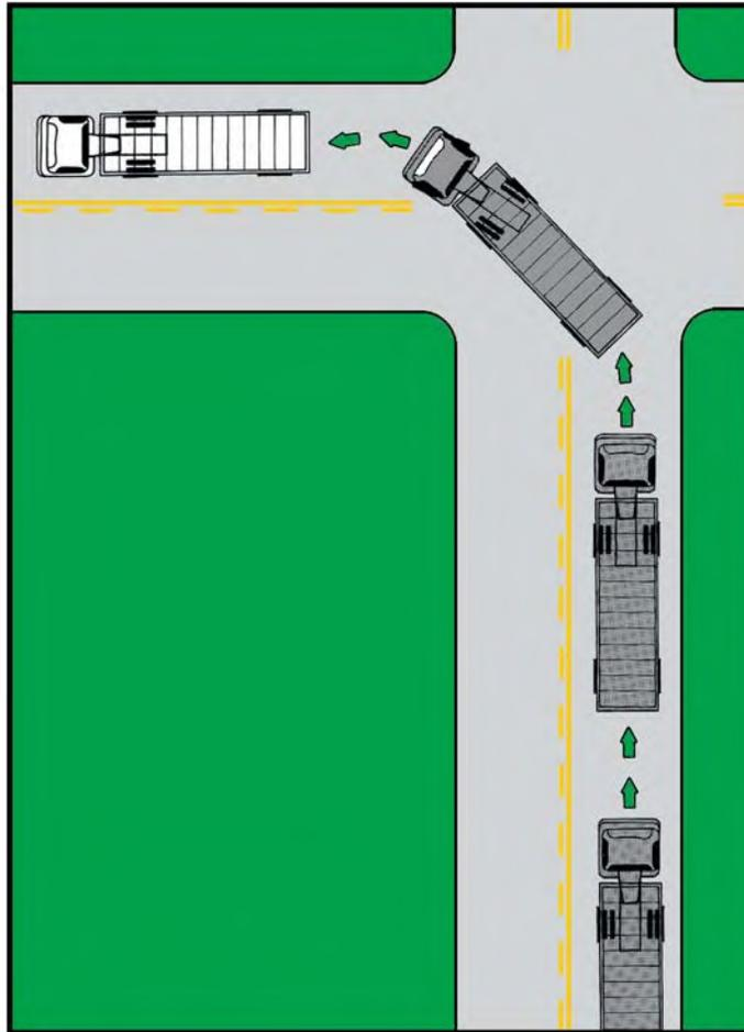
This illustration is the correct procedure for making a left turn with a tractor semi-trailer. The procedure is the same with a single-unit vehicle.
