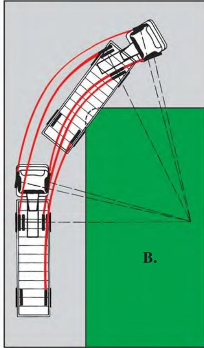
In illustration B, notice the rear wheels of the trailer follow shorter paths than the front wheels of the tractor.
